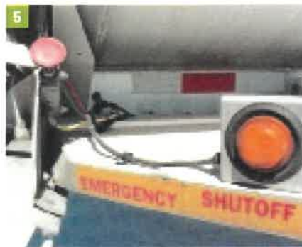
(4) A cable device that is operated by pulling on the red latch. (5) A pneumatic device that is operated by pressing on the round red plunger at the left.
