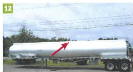
(11) A vent hole between a double bulkhead. (12) A typical MC-406 tanker trailer. Along the top is the eight-inch overturn protection rail (arrow) through which runs the vapor recovery system and the access ladder at right.
