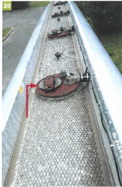
(20) On the manhole, clockwise from left (arrow) are the dome hatch, the Scully device, and the vapor valve.
