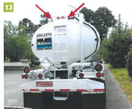
(13) From the rear, note the elliptical shape, the ladder, and the vapor recovery piping. This tanker has baffle holes in the 3 and 6 o'clock positions, as indicated by the black dots. This allows liquid to flow to both sides of the baffle when the tanker is on its side. Also note the water drain hoses (arrows) connected to the hollow ladder rail, as described previously.
